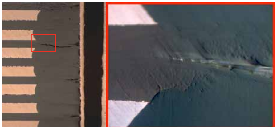
Figure 3. Void/delamination from resin starvation is linked to cracks emanating from the copper foil.
