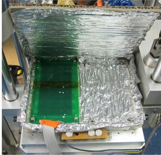
The PCBA was designed to include a controlled impedance trace throughout the PCB such that controlling the current flow through the trace would directly impact its thermal dissipation. An external controller circuit with a thermocouple feedback loop was designed to control the localized temperature of the board (set to 125C) and the components soldered to it.
