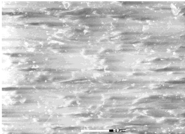
Figure 3 (320x): SEM cross-sectional view showing an enlarged image of the inner core of the CEM substrate.
