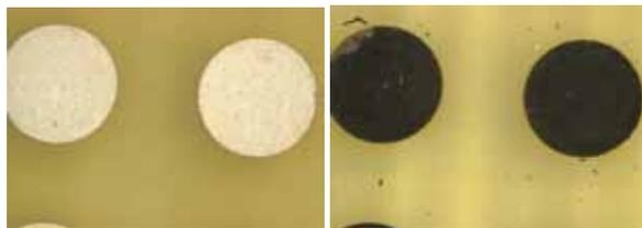
**Figure 4:** Immersion silver coupons before (left) and after (right) eight days of exposure to Class II MFG conditions
