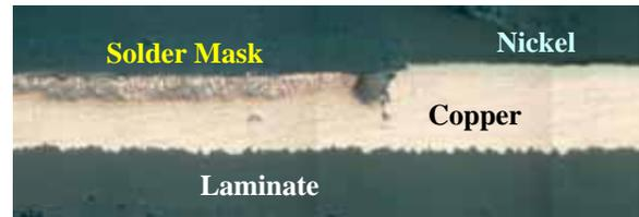
**Figure 17:** Optical micrograph of cross-section of ENIG-plated bond pad experiencing crevice corrosion
