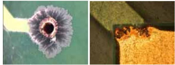
**Figure 16:** Optical micrographs of corrosive growths observed on ENIG-plated PCBs
