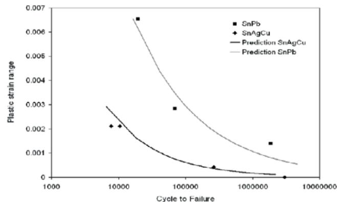
Figure 3: Vibration behavior of SAC solder
