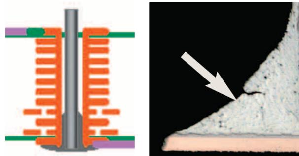
Figure 4: Examples of insufficient hole fill and fillet cracking
