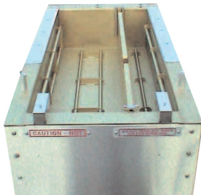
The I.R. preheater is best when used in conjunction with a forced air convected preheater. The force air convected preheater acts as heater for the topside of the PCB. Lead-free solders do not seem to flow up thru-holes as easily as leaded solders. Topside preheat will allow better process control, giving the operator the ability to more accurately control the temperature of the topside of the board.
