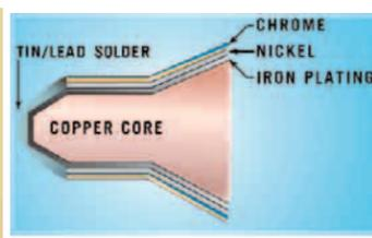
Cross-section of typical solder tip, with lead-free the solder is lead-free
