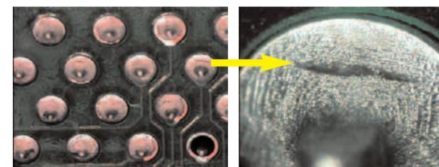
Solder shrinkage effects on solder joints.
