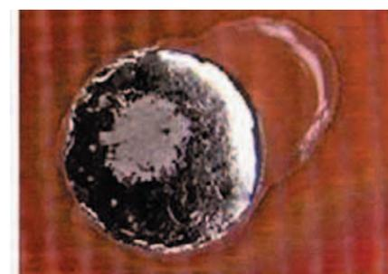
Figure 1. Lead Free Solder Joint with Flux Residue
