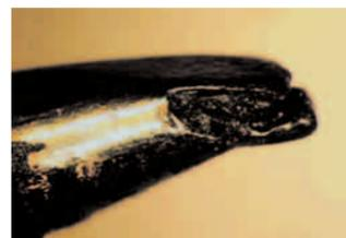
Lead-free tip failure after 3 weeks
