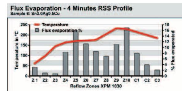
Figure 2. Ramp Soak Spike Profile
