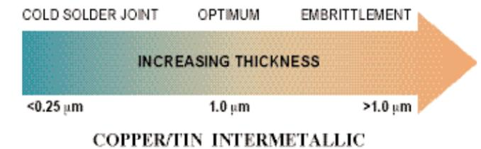
Higher temperatures and longer contact with the parts to be soldered may also increase the intermetallic bond layer. So avoiding prolonged contact and repeated rework is not recommended. The above diagram shows what happens as the bond layer increases in thickness a higher risk of embrittlement occurs.
