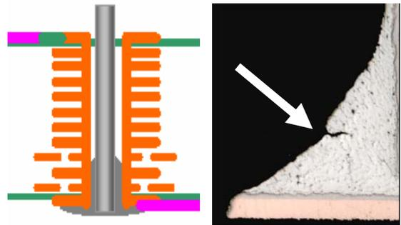
Figure 5: Examples of insufficient hole fill and fillet cracking
