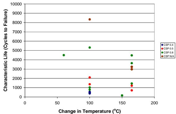
**Figure 8:** Cycles to failure as a function of change in temperature during thermal cycling for CSPs attached with SAC solder. Coloration identifies different pitches (0.4 mm, 0.5 mm, 0.8 mm, unknown).
