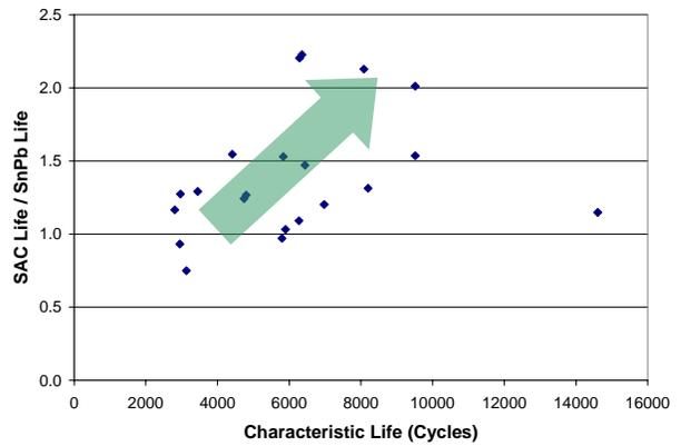
**Figure 14:** Ratio of SAC/SnPb reliability for area array devices as a function of characteristic lifetime of the SAC component.
