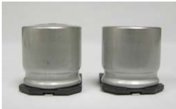
Figure 1: Aluminum liquid electrolytic capacitor, on the left-hand side, that has experienced case distortion after an extended time at Pb-free reflow temperatures
