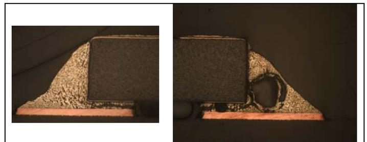
**Figure 5:** Optical micrographs of cross-sectioned 2010 chip resistor solder joints after exposure to 1800 hours of temperature cycling (see Figure 1).
