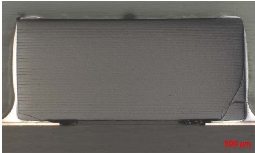
Figure 14: Flex cracking in a capacitor
