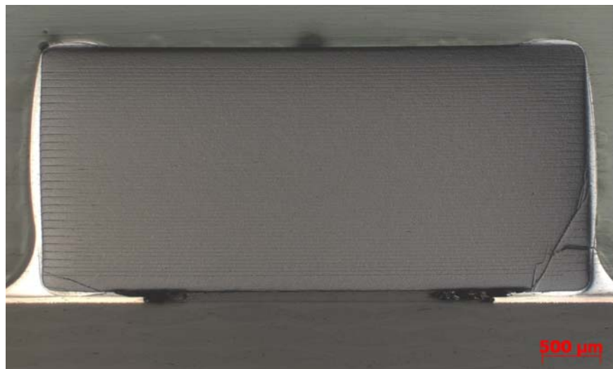
Figure 14: Flex cracking in a capacitor
