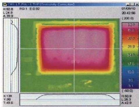
Fig. 7. Thermal image of front panel (IR measurement).
