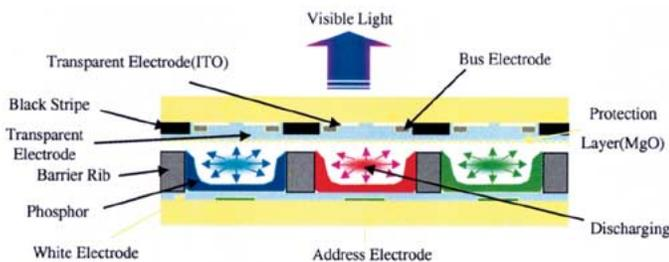
Fig. 2. Cross section of plasma display panel.
