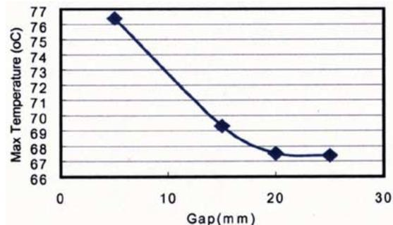
Fig. 19. Maximum temperatures versus gap.
