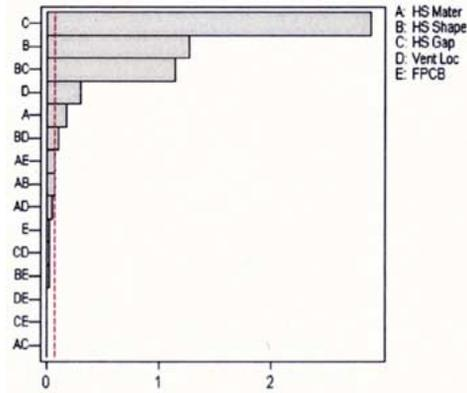
Fig. 17. Pareto chart of the effects (Response is max temperature).
