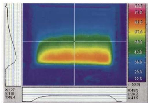
Fig. 12. Measured temperature distribution at white/black pixel.
