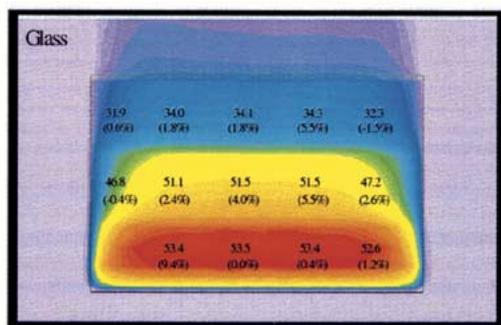
Fig. 10. Simulated temperatures on front panel at white/black pixel.
