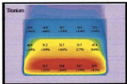
Fig. 11. Simulated temperatures on back panel at white/black pixel.
