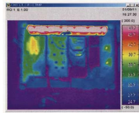
Fig. 8. Temperature map of backside of PDP (IR measurement).
