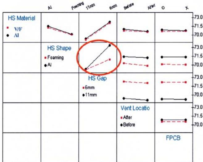
Fig. 15. Interaction plot for response (max. temperature °C).
