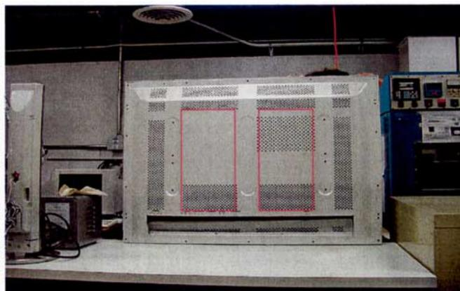
Fig. 13. Vent location (dots-before, red line-after).
