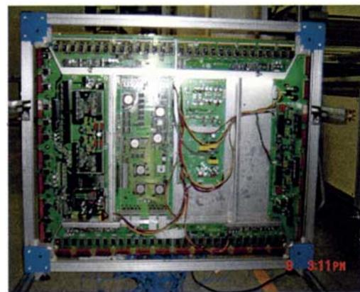
Fig. 5. PCBs on back of PDP.
