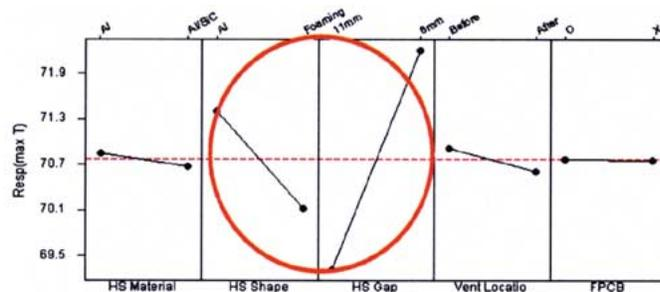
Fig. 14. Main effect plot for response (max. temperature °C).
