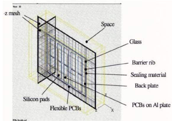
Fig. 4. Components of the simulation model.
