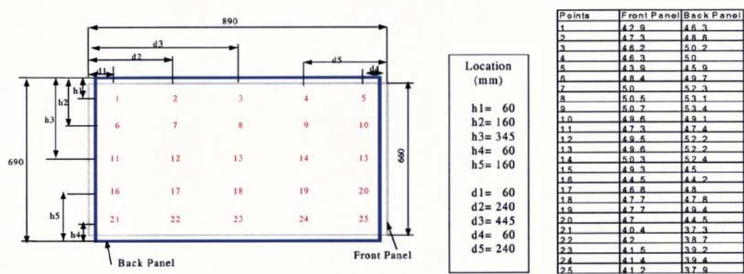
Fig. 9. Location of temperature measurement points and measured data.
