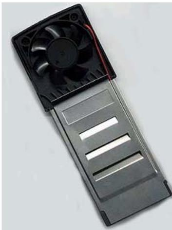
**Figure 5:** PCMCIA fan for supplemental cooling
