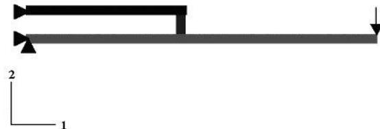
**Figure 4:** FEA beam model of 0805 capacitor
