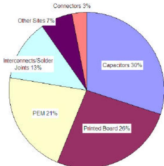
**Figure 1:** Field failure occurrence by failure site
