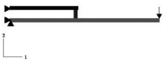
**Figure 5:** FEA beam model of 0805 capacitor
