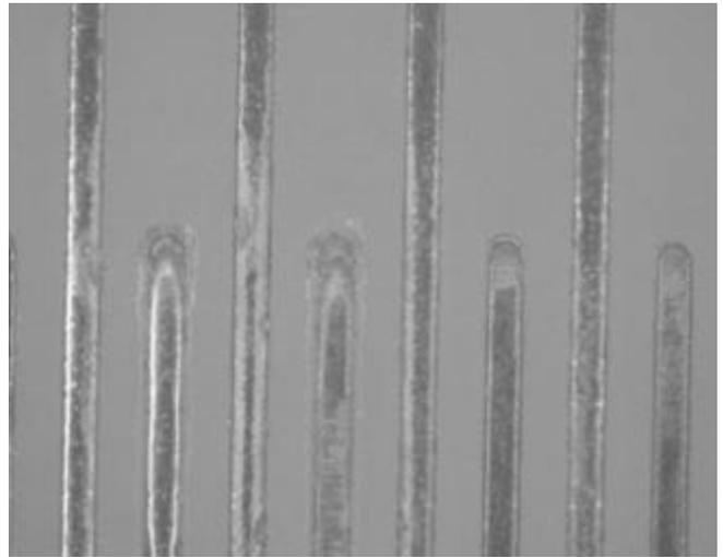
**Figure 5. Uniform corrosion on 6.25 mil spacing at 5 mg/in<sup>2</sup> Cl.**
