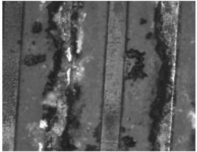
**Figure 4. Uniform corrosion on 6.25 mil spacing at 50 mg/in<sup>2</sup> Cl.**
