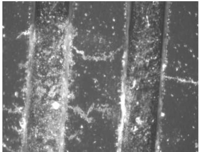
Figure 2. Dendritic growth on 6.35 mil spacing at "0" mg/in<sup>2</sup> Cl.
