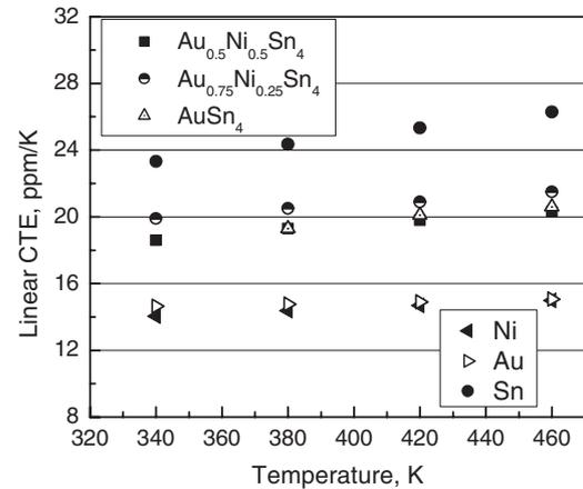
Fig. 2. Linear CTEs for  $\text{Au}_{0.5}\text{Ni}_{0.5}\text{Sn}_4$ ,  $\text{Au}_{0.75}\text{Ni}_{0.25}\text{Sn}_4$ , and  $\text{AuSn}_4$  (see also Table 5). Literature data for Ni, Au, and Sn metals [15] are also shown.
