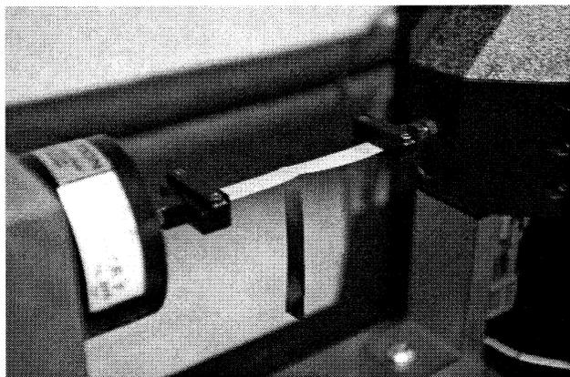
Fig. 1. T-peel test for evaluation of adhesive strength.
