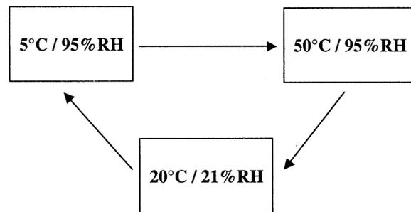
Fig. 6. Temperature/humidity cycling conditions.
