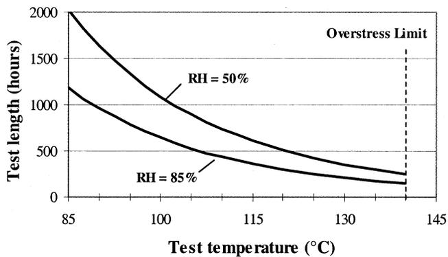
Fig. 5. Aging test length as a function of temperature and humidity settings.
