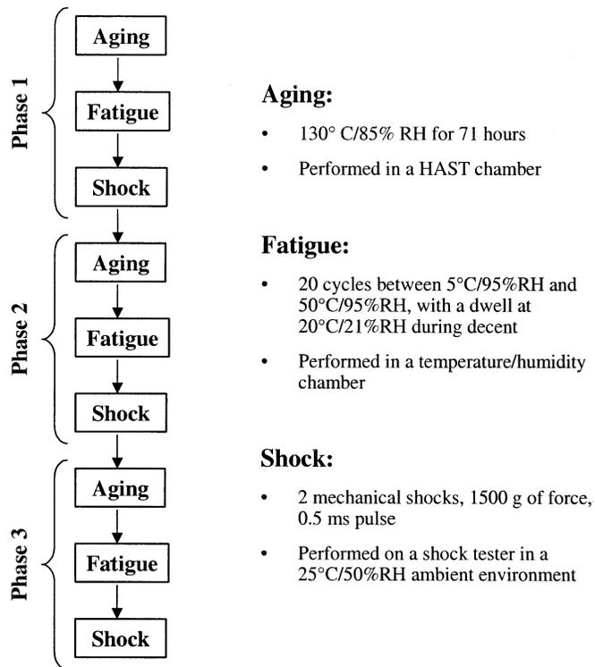
Fig. 7. Test flow for SPIE deadhesion test.
