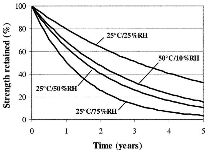
Fig. 4. Predicted degradation of SPIE at various application conditions.
