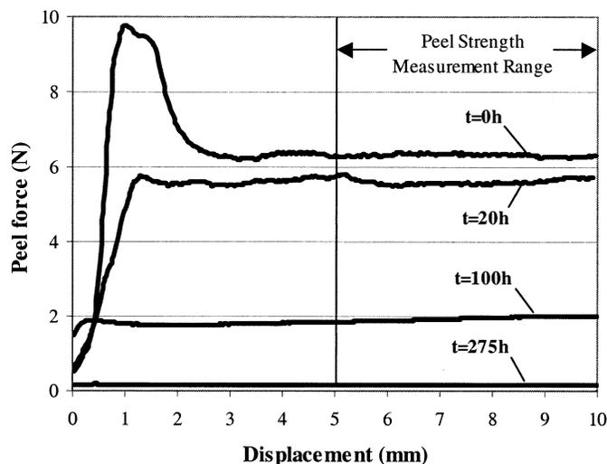
Fig. 2. Peel strength test results for a sample aged at 130 °C/85%RH.
