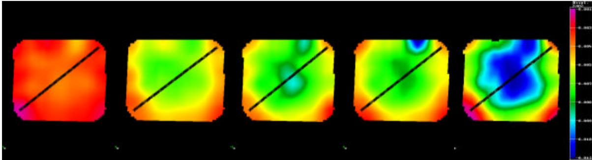
Figure 3. Series of Images with Fixed Scale Showing Progression of Warping during Cool-down Process.
