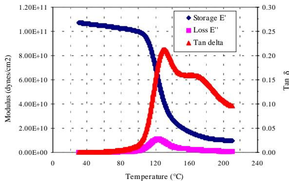
Figure 1. Viscoelastic Modulus of Plastic Molding Compound
