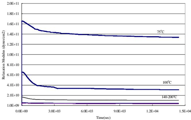
Figure 11. Relaxation Modulus of 0.25% Strain Application at 75-200°C
