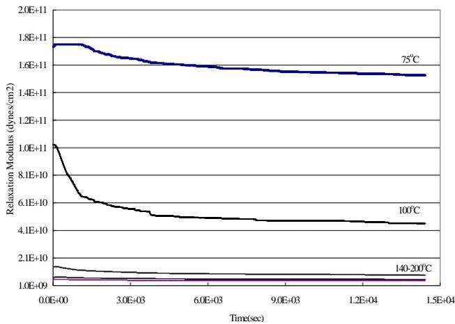
Figure 10. Relaxation Modulus of 0.1% Strain Application at 75-200°C
