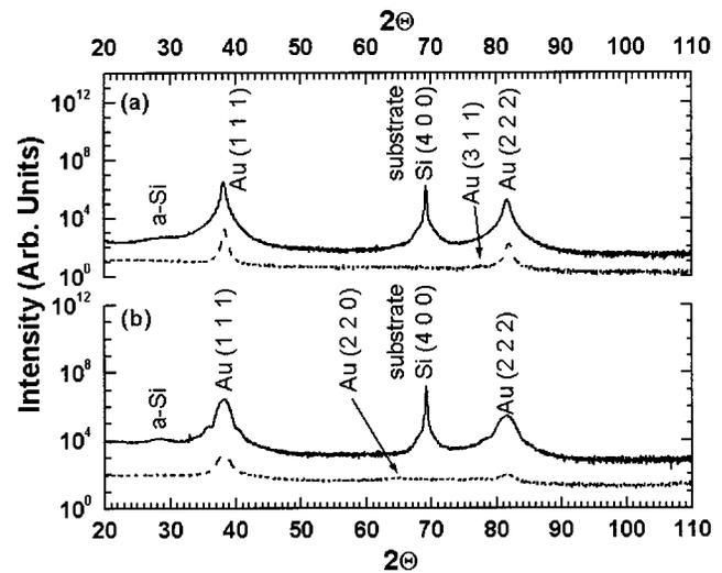
FIG. 1. X-ray diffraction data for as-prepared Au/*a*-Si multilayers of two different modulations,  $\lambda = 47$  nm (a) and  $\lambda = 14$  nm (b). Dashed curves are for samples prepared on NaCl substrates and solid curves are for samples prepared on Si(100). The samples exhibited a (111) preferred orientation for Au and the typical broad peak for amorphous Si at approximately  $28.5^\circ$ .
