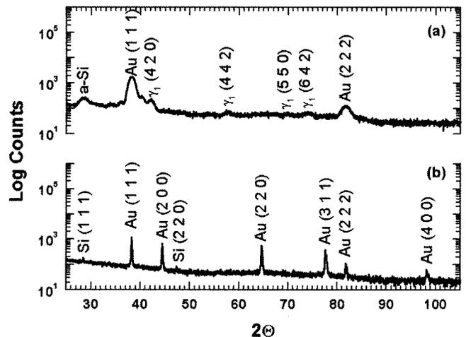
FIG. 7. X-ray diffraction data for samples with a modulation of  $\lambda = 14$  nm that were heated to intermediate temperatures [453 K (a) and 623 K (b)] in a differential scanning calorimeter and then quenched to room temperature.
