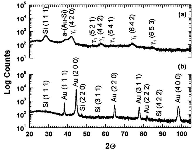
FIG. 6. X-ray diffraction data for Au/a-Si samples prepared with a modulation of  $\lambda = 6.1$  nm that were heated to intermediate temperatures [462 K (a) and 648 K (b)] in a differential scanning calorimeter and then quenched to room temperature.
