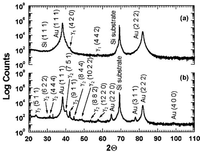
FIG. 4. X-ray diffraction data for Au/a-Si multilayers ( $\lambda = 47$  nm) annealed at 423 K (a) and 523 K (b). Evidence is found for the formation of the  $\gamma_1$  phase for the lower temperature anneal, and the formation of a second metastable silicide, identified as the  $\gamma_2$  phase (Ref. 21), at higher temperatures.
