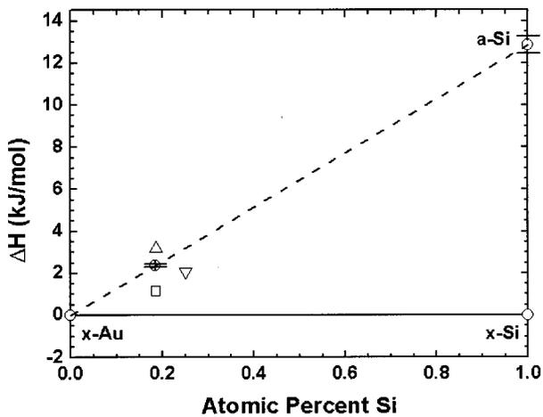
FIG. 8. A plot of the enthalpy of formation vs atomic percent Si for the Au–Si system. Data are plotted for the enthalpy of formation for pure elements and *a*-Si (O). The dashed line represents the enthalpy for a phase mixture of Au and *a*-Si. Three measurements are also plotted for the enthalpy of formation of metastable silicides: Chen and Turnbull ( $\Delta$ ) (Ref. 19), Gnauert ( $\nabla$ ) (Ref. 29), and the measurement made here ( $\square$ ).
