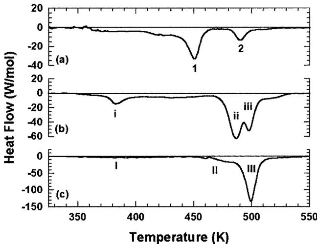
FIG. 5. Heat flow vs temperature measured by differential scanning calorimetry for Au/a-Si multilayers prepared with three different modulations:  $\lambda = 6.1$  nm (a),  $\lambda = 14$  nm (b) and  $\lambda = 47$  nm (c).
