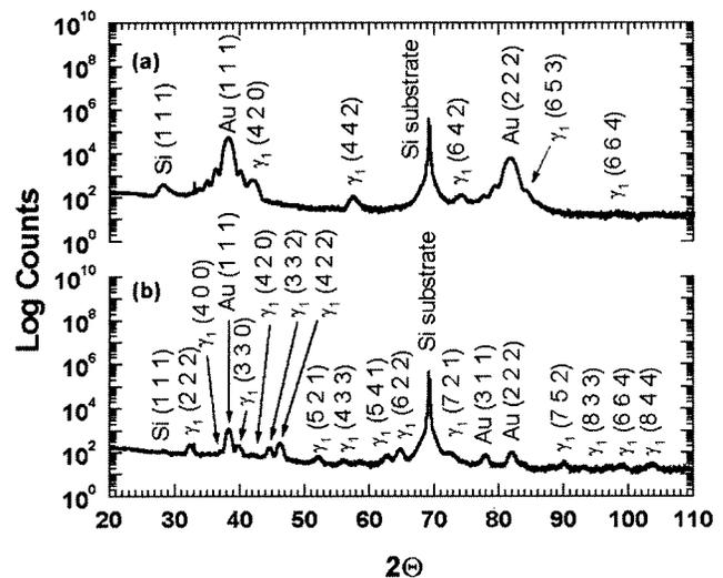
FIG. 3. X-ray diffraction data for Au/*a*-Si multilayers ( $\lambda = 14 \text{ nm}$ ) prepared on Si (100) and annealed at 423 K (a) and 513 K (b). Evidence is found for the growth of the  $\gamma_1$  phase identified by Krutenat *et al.* (Ref. 18) at both temperatures.
