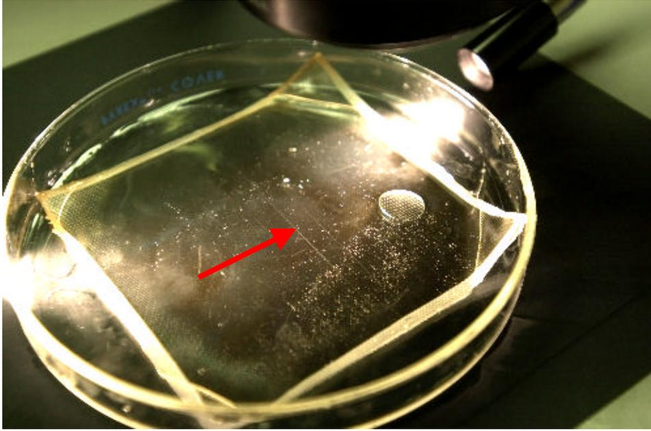
**Figure 3.** A change in the refractive properties is evident through an optical microscope by a bright white line. In this case, a hollow can be detected with the unaided eye (see red arrow). They usually span the entire length of the laminate and may also weave back and forth.
