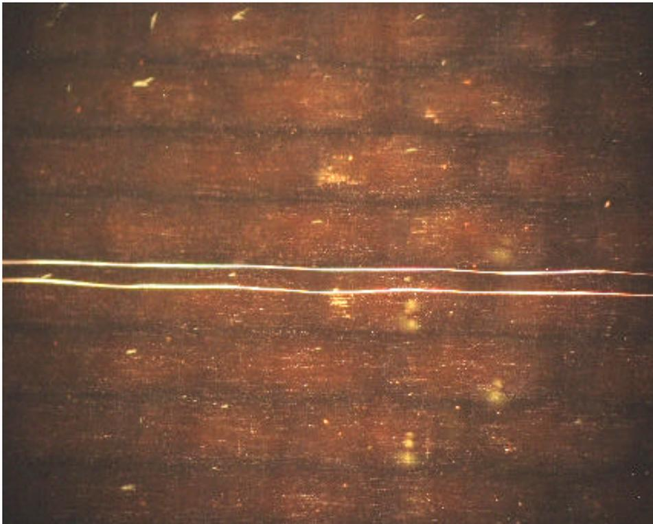
**Figure 4.** Two hollow fibers can be seen as bright white lines traversing the horizontal direction. They usually span the entire length of the laminate and may also weave back and forth. Therefore, some of the hollow fibers that run in the same direction may in fact be connected and due to the same trapped air bubble. Magnification = 50X
