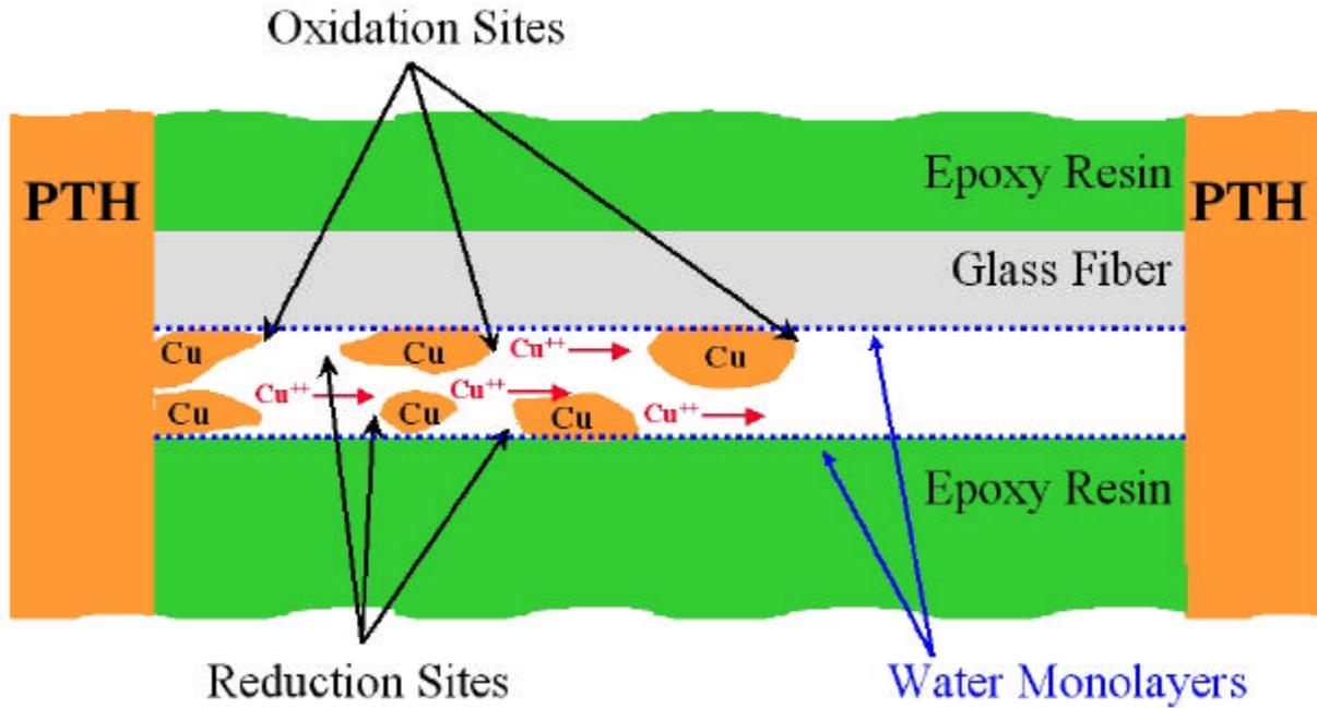
**Figure 1.** The most common corrosion path for CFF is between a glass fiber and the epoxy resin. Once this delamination occurs, next step is the introduction of the electrolyte – water. When the moisture level increases, an oxidation reaction will occur, forming copper ions, which under bias will migrate towards the negatively biased conductor.
