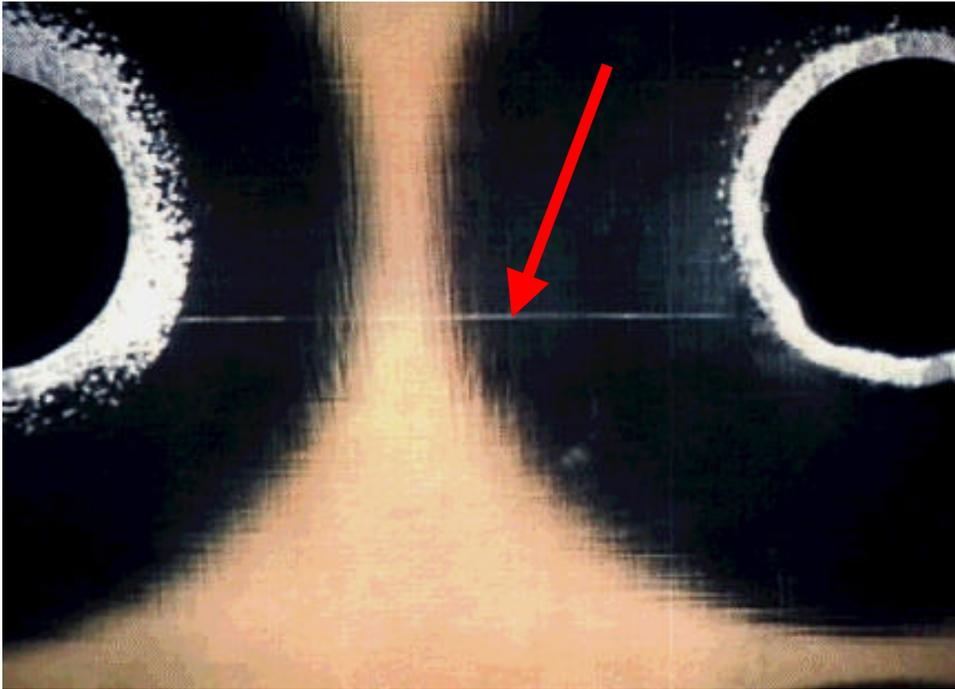
Figure 6. This hollow fiber, seen as a bright white line traversing the horizontal direction (see arrow), was responsible for failure of this PWB assembly by causing a short between the two conductors it electrically connected. Magnification = 125X
