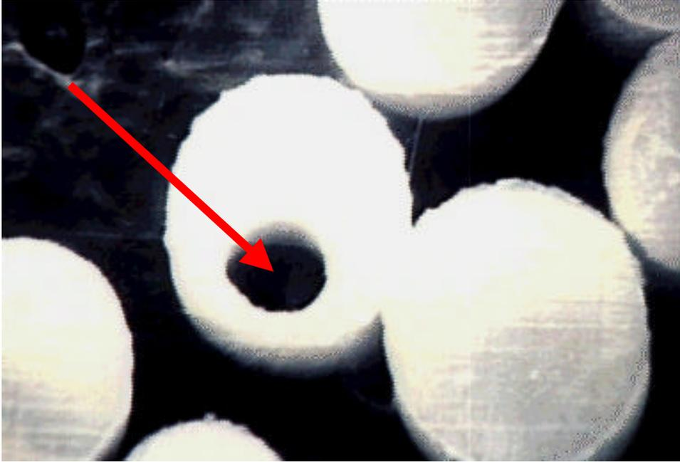
Figure 5. A cross-section of a hollow fiber can be seen in the middle fiber in this photo. Magnification = 6000X
