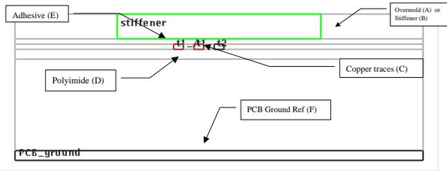
Figure 8. Basic cross section for electromagnetic analysis.
