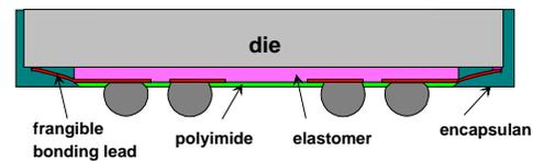
the shear strain caused by the thermal expansion mismatch between the silicon die and the circuit board substrate.
