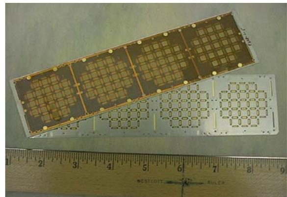
Figure 4. Cavity-Up Enhanced BGA substrate of 7mm (64 I/O) packages at 0.5 mm ball pitch in a 4 in array format yielding 84 packages per substrate.
